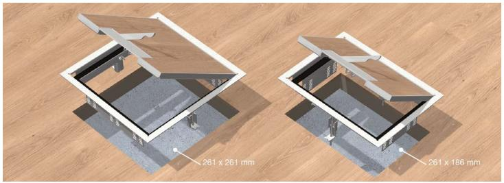
Quadrangular cartridge installation units with carpet protection frame made of high-grade steel with outer measurements of 284x284 mm or 284x211 mm for the installation in hollow space floors or raised floors. For parquet flooring of 12/22 mm.
