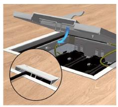
**5 | Axis**Open the cable outlet with the opening lever and swivel the cable outlet axis.
