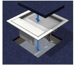
**1 | Unit**For the installation of a device cup, place cartridge unit UEKDD1-2 V E into the opening.
