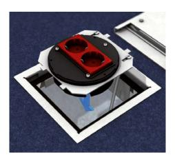
5 | Inserting of device cup Insert plate with the pre-mounted and loaded device cup through the plate slide as deep into the lock-in leads in the frame as possible. A gradual lowering of the plate to max 20 mm possible.
