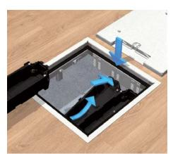
**4 | Rubber seal / Device cup**Glue the rubber seal to the impact-noise interface. Snap the device cup as deep into the lock-in leads as possible. When using an device plug H = 35 mm, the minimum installation depth is Hmin = 91 mm.
