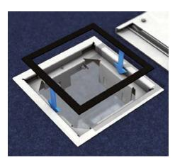
**4 | Rubber seal**Glue the rubber seal for impact-noise decoupling into the frame.
